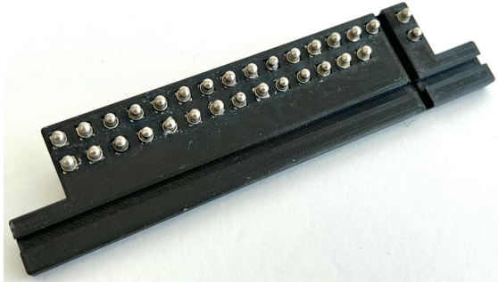
Pic. 13a: 3D printed bracket with spring contacts
